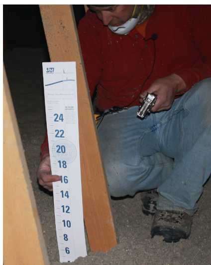
Figure 1. Measuring attic insulation thickness.
