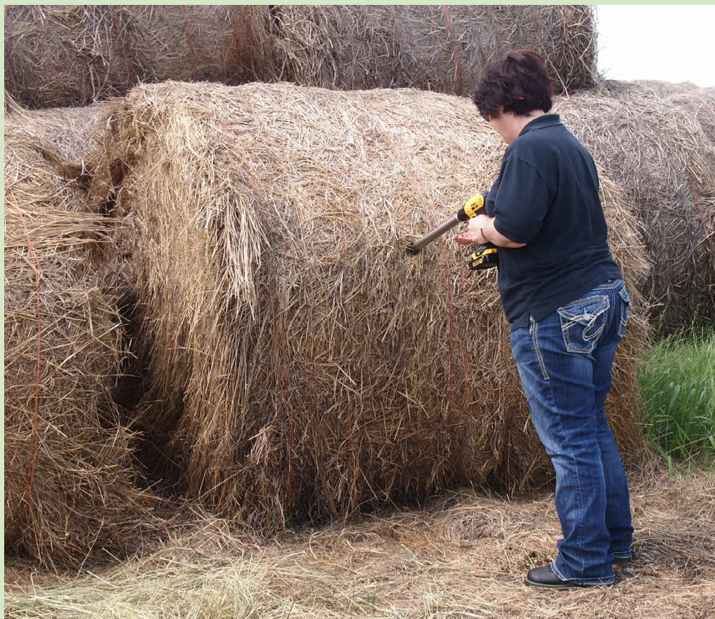
Figure 1. Forage sampling a round bale using a Penn State sampler with an electric drill.
