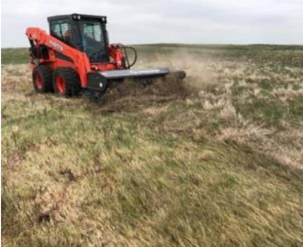
**Figure 2a:** An 82-inch Titan Implement Xtreme Skid-Steer Angle Broom Attachment connected to an SSV75 Kubota Skid-Steer used to remove bluegrass thatch and litter from plots. Photo by Hayley Hilfer
