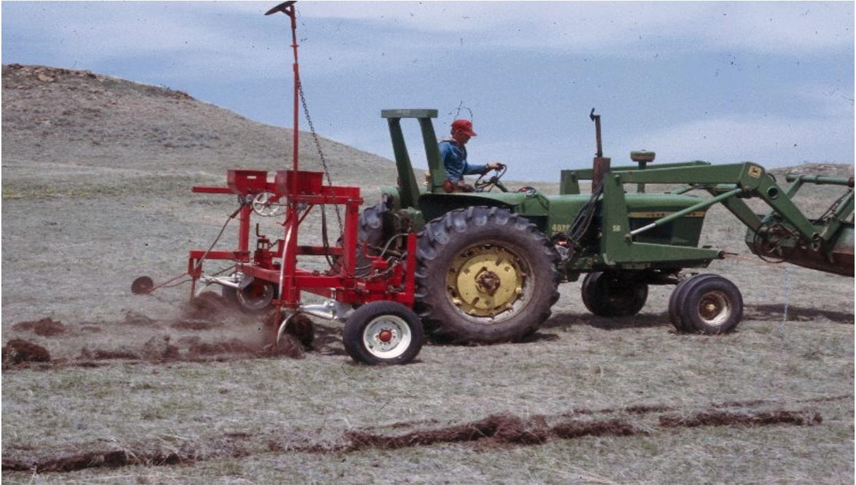
**Fig. 3. Interseeding machine with two shanks at ten-foot row spacings.**
