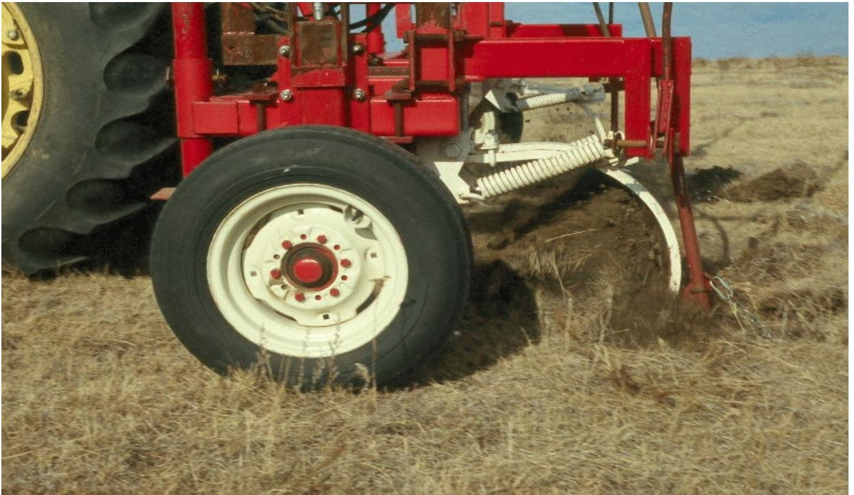
**Fig. 4. Interseeding machine at ten-foot row spacings.**
