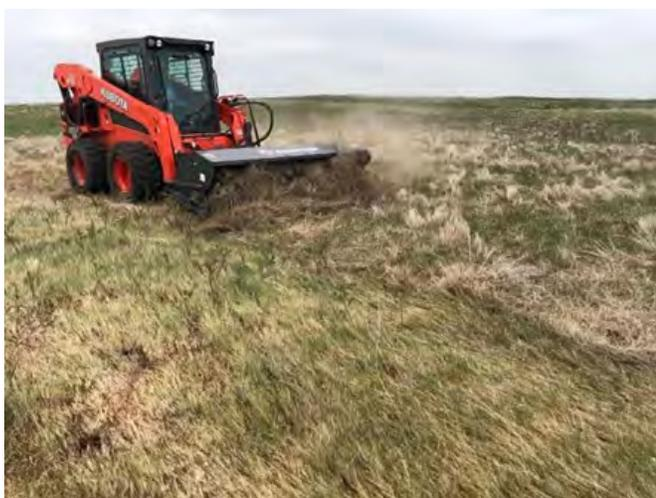
**Figure 2a.** 82-inch Titan Implement X-treme Skid-Steer Angle Broom Attachment connected to a SSV75 Kubota Skid-Steer.
