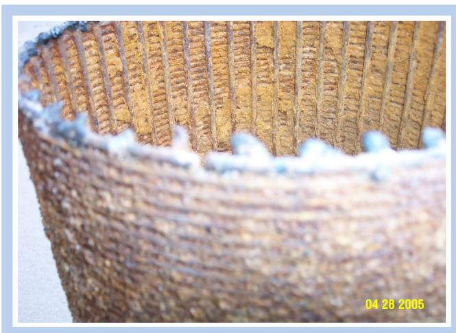
Figure 6. Encrusted minerals on the inside of a totally plugged well screen.
