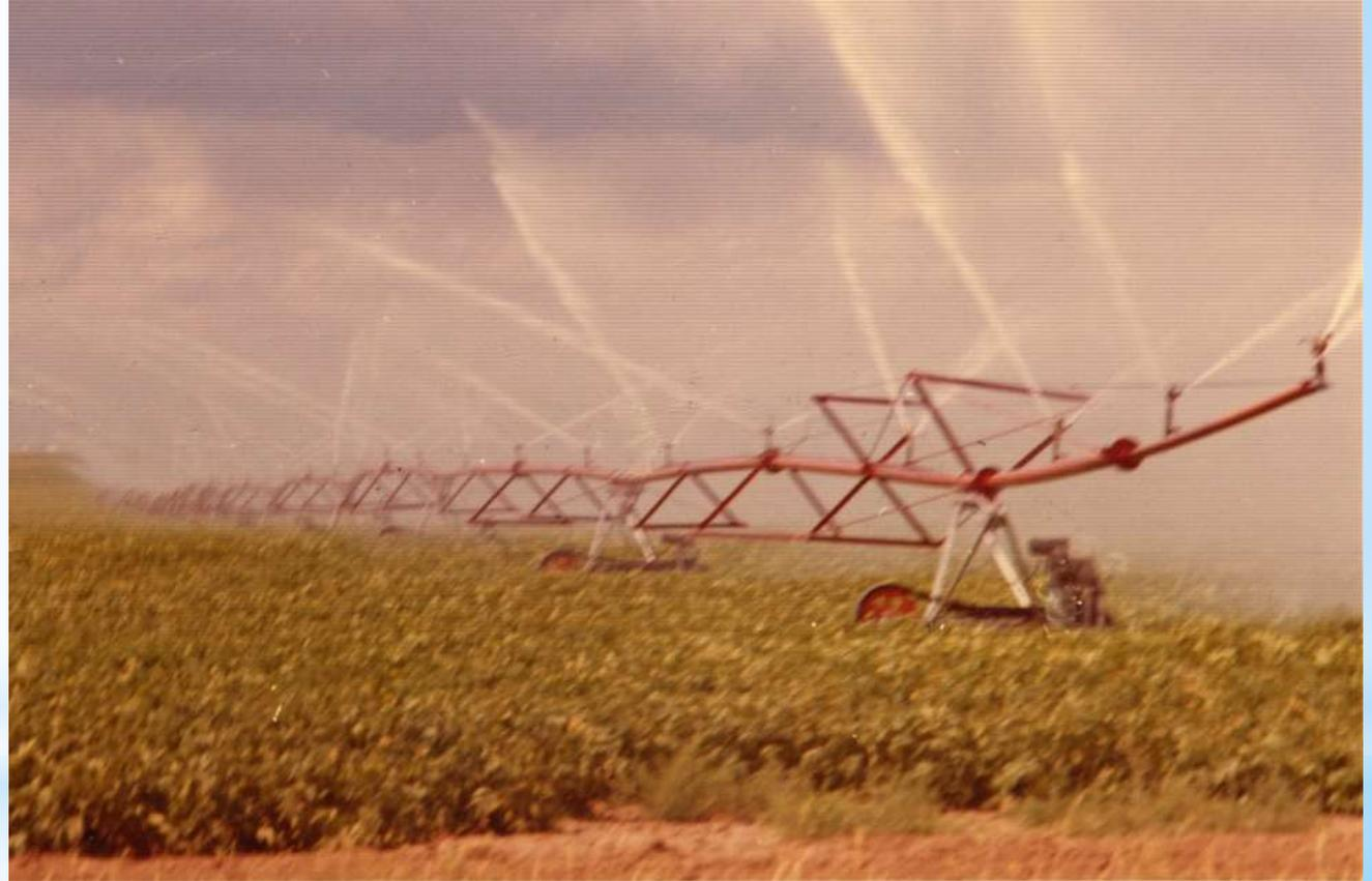
Another development in the 1970's was the "lateral move" (sometimes called a linear move) irrigation system. It uses the same structural design as a center pivot, but all the towers move in unison across the field. This is a modern, low-pressure system located in the Nesson Valley east of Williston, ND.
