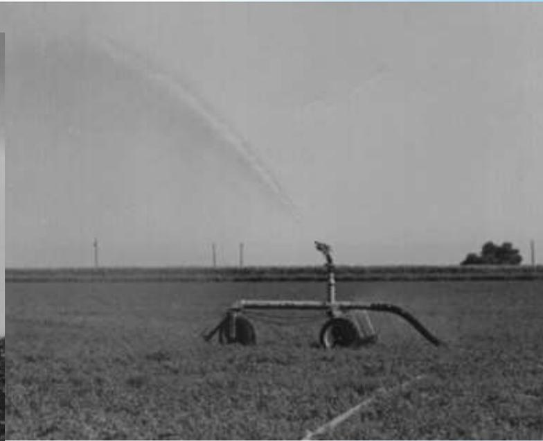
Volume sprinklers (commonly called “Big Guns”) have been used from the 1950’s up to the present day. They can throw water from 150 to 300 feet depending on nozzle size, pressure at the sprinkler head and angle of throw.
