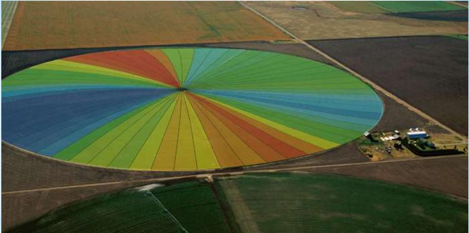
Modern center pivots are now being used for “precision application of water.” This management option (shown above) changes the application amount by varying the speed of the center pivot.
